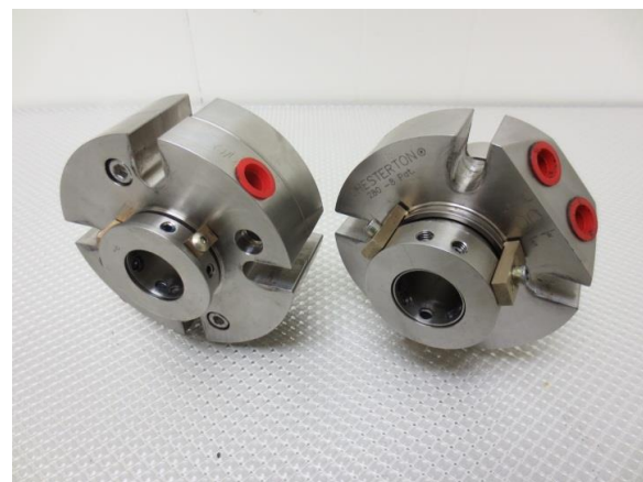
FIGURE 3: THE CHESTERTON 180 HEAVY DUTY CARTRIDGE SINGLE SEAL (LEFT) AND THE CHESTERTON 280 HEAVY DUTY CARTRIDGE DUAL SEAL (RIGHT) TESTED IN THIS STUDY [12].
