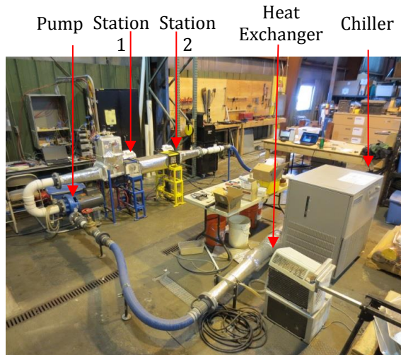
FIGURE 1: VIEW OF THE ENTIRE FLUME.
