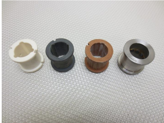
FIGURE 4: THE FOUR CANDIDATE BEARINGS TESTED IN THIS STUDY, FROM LEFT TO RIGHT - VESCONITE, CIP MARINE, FEROFORM T814, AND POLYCRYSTALLINE DIAMOND (PCD) RADIAL BEARING [12].
