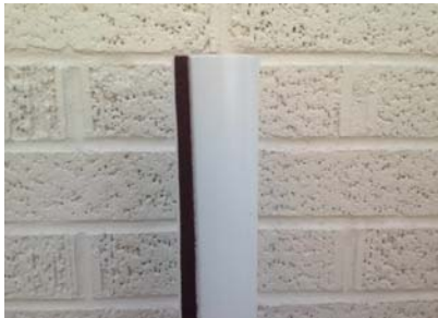
FIGURE 4. CYLINDER WITH THE P60 STRIP ATTACHED AT 60^\circ FROM THE STAGNATION POINT.
