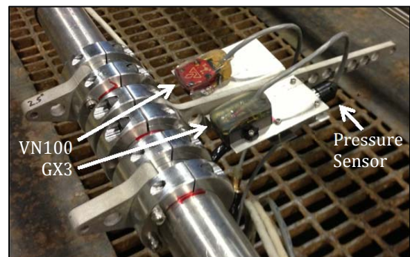
FIGURE 10. INERTIAL MEASUREMENT UNITS AND PRESSURE SENSOR
