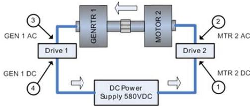
**FIGURE 13: SETUP FOR BACK-TO-BACK TESTING OF GENERATOR-DRIVE**
