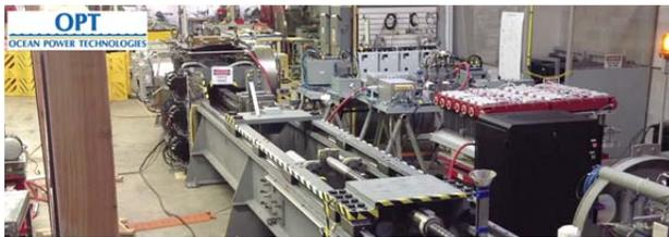
**FIGURE 15: PTO ENDURANCE TEST SETUP AT OPT**
