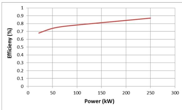
**FIGURE 16: MEASURED MECHANICAL TO ELECTRICAL PTO EFFICIENCY**
