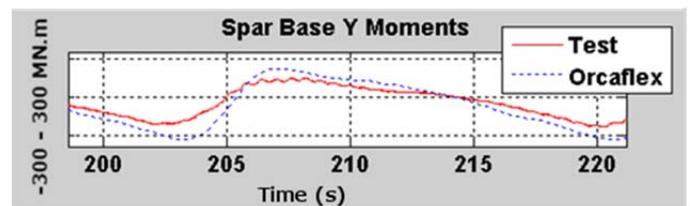
FIGURE 4: EXAMPLE OF ORCAFLEX MODELING OF SPAR LOADS
