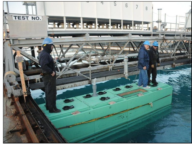
FIGURE 7. "RHO-CEE" MODEL BEING PREPARED FOR ABSORPTION TESTS AT OHMSETT FACILITY.
