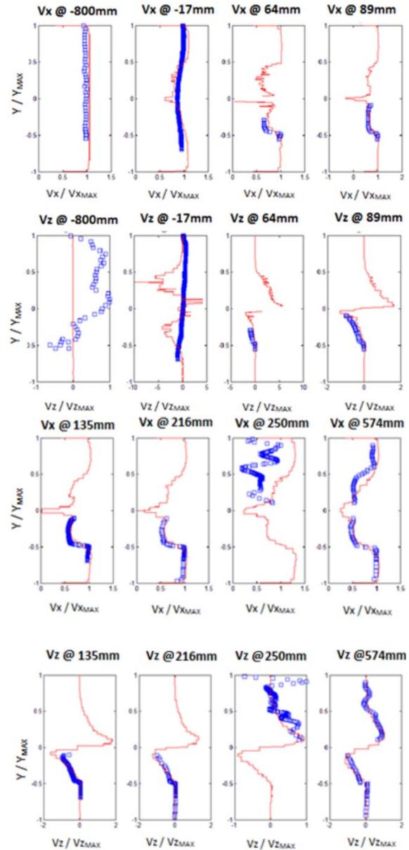
**FIGURE 4. COMPARISON OF MEASURED (BLUE) AND SIMULATED (RED) STREAMWISE ( $V_x$ ) AND VERTICAL ( $V_z$ ) VELOCITIES AT DIFFERENT CROSS-SECTIONS. LOCATIONS ARE SHOWN AS DISTANCES FROM THE TURBINE ROTOR PLANE WITH THE NEGATIVE SIGN INDICATES LOCATION UPSTREAM OF THE TURBINE.**
