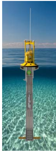
FIGURE 1: SCHEMATIC OF APB CONSISTING OF SURFACE FLOAT, SPAR CONTAINING POWER TAKEOFF, AND HEAVE PLATE CONSTRAINING SPAR MOTION
