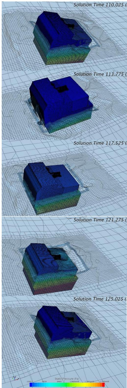
**FIGURE 1: SNAPSHOTS FROM A SINGLE WAVE PERIOD OF BBDB SUBJECTED TO EXTREME SEA STATE.**
