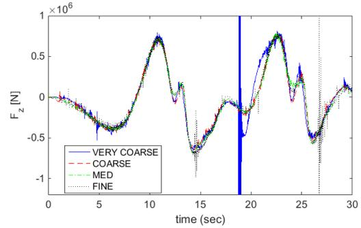
FIGURE 7: MODEL WEC PTO HEAVE FORCE (CONVERGENCE) PLOT.
