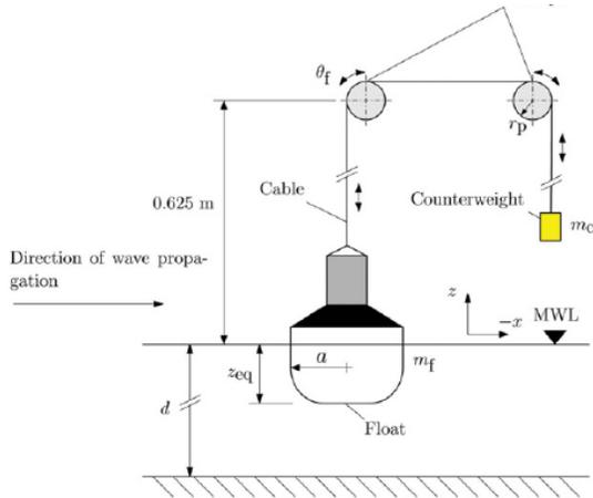
FIGURE 2: DIAGRAM OF BOBBER TEST [4]
