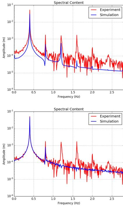
Figure 3: Comparisons of simulation to experimental FFTs for  $h = 1.0, 0.25$  (top to bottom) and  $\Delta t = 0.02$  s.
