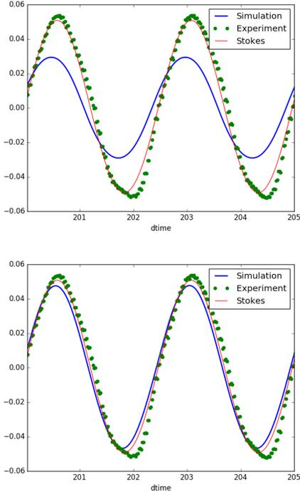
Figure 1: Comparisons of simulation to experimental results for  $h = 1.0, 0.25$  (top to bottom) and  $\Delta t = 0.02$  s.
