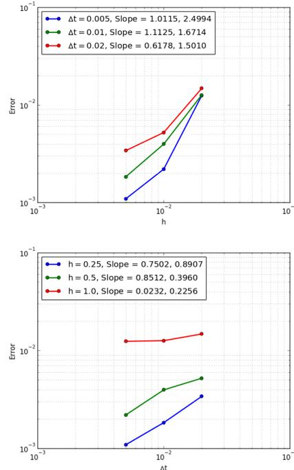
Figure 5: Numerical error vs  $h$  (top) and  $\Delta t$  (bottom) for each temporal discretization
