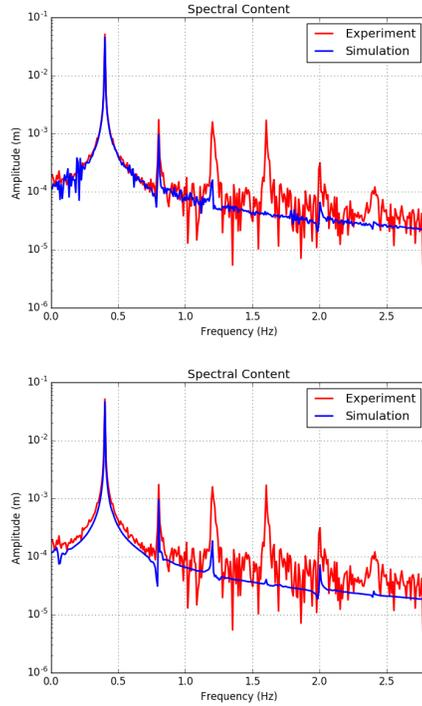
Figure 4: Comparisons of simulation to experimental FFTs for  $h = 0.5$  and  $\Delta t = 0.02, 0.05$  s (top to bottom).
