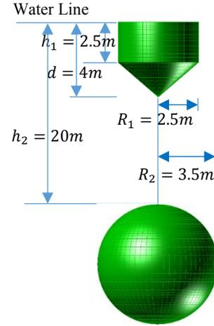
**Figure 3.** Dimension and mesh of the self-reacting wave energy converter used for WAMIT
