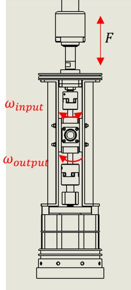
**Figure 2.** Schematic of the power takeoff system with mechanical motion rectifier
