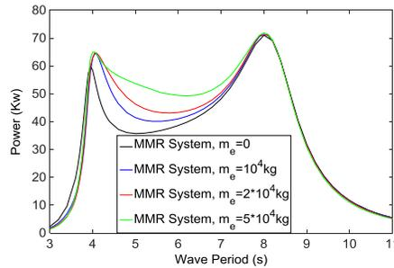
**Figure 5.** Optimum power of the MMR system with various designs of equivalent mass  $m_e$  under regular wave excitation. The wave height is 2m.  $c_{d2}$  is 0.5.
