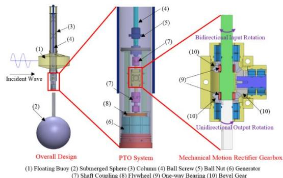
**Figure 1.** Configuration of the proposed self-reacting wave energy converter with mechanical power takeoff system
