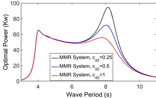
**Figure 6.** Optimum power of the MMR system with various selection of drag coefficient  $c_{d2}$  under regular wave excitation. The wave height is 2m.
