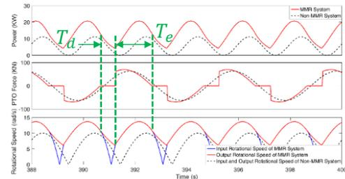
**Figure 4.** Simulation results of a self-reacting wave energy converter for MMR system and Non-MMR system under regular wave excitation.  $T_d$  and  $T_e$  are the disengagement and engagement periods.
