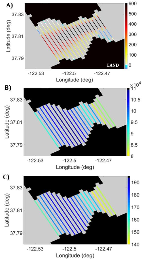
**FIGURE 3: RESULTING A) DISCRETE  $Q_i^{(2)}$  ( $m^3/s$ ), B) TOTAL  $Q_{MAX}$  ( $m^3/s$ ), AND C)  $P_{MAX}$  (MW) IN SAN FRANCISCO BAY FROM VELOCITY CALCULATION METHOD 2, WHICH INCORPORATES CONSTITUENT INCLINATION ANGLE BUT DOES NOT ACCOUNT FOR CONSTITUENT PHASE**
