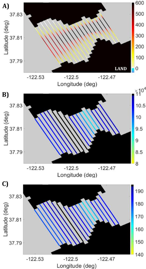
**FIGURE 2: RESULTING A) DISCRETE  $Q_i^{(1)}$  ( $m^3/s$ ), B) TOTAL  $Q_{MAX}$  ( $m^3/s$ ), AND C)  $P_{MAX}$  (MW) IN SAN FRANCISCO BAY FROM VELOCITY CALCULATION METHOD 1, WHICH DOES NOT INCORPORATE CONSTITUENT INCLINATION ANGLE NOR PHASE**
