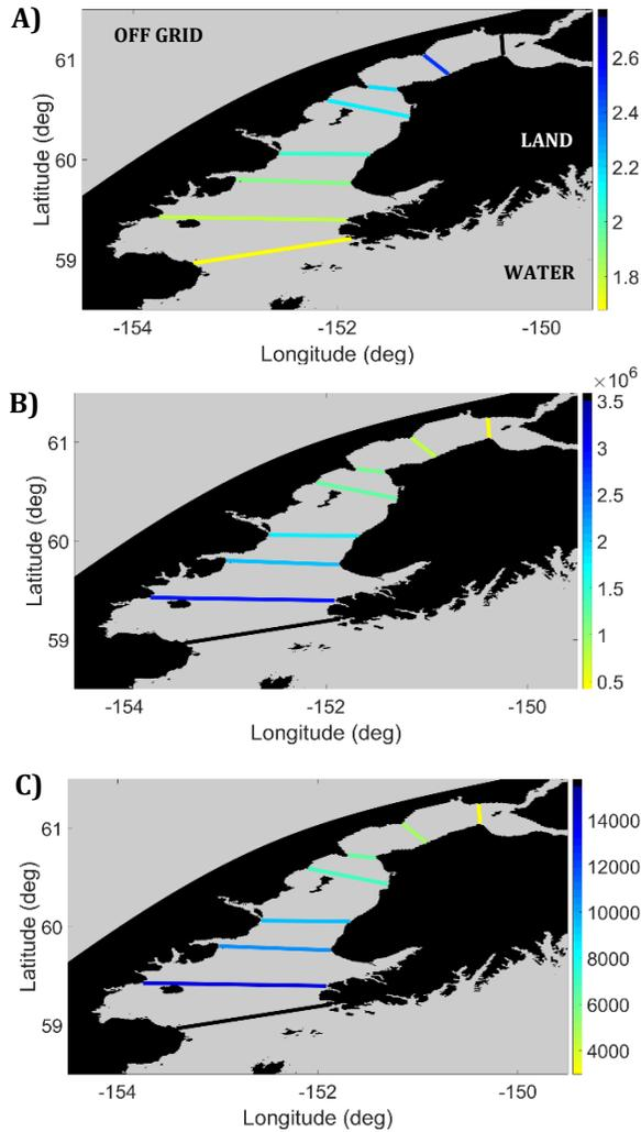
**FIGURE 5: SPATIAL VARIATION OF A) M2 AMPLITUDE, B)  $Q_{MAX}$ , AND C)  $P_{MAX}$  IN COOK INLET, AK, USA**
