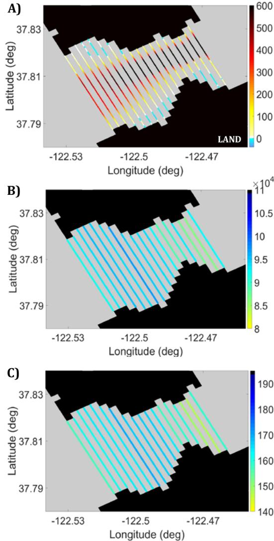
**FIGURE 4: RESULTING A) DISCRETE  $Q_{i,t,max}^{(3)}$  ( $m^3/s$ ), B) TOTAL  $Q_{MAX}$  ( $m^3/s$ ), AND C)  $P_{MAX}$  (MW) IN SAN FRANCISCO BAY FROM VELOCITY CALCULATION METHOD 3, WHICH INCOPORATES BOTH CONSTITUENT INCLINATION ANGLE AND PHASE**
