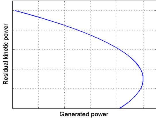
**FIGURE 1: ILLUSTRATION OF THE EFFECT OF DIMINISHING RETURNS FROM ADDING ADDITIONAL TURBINES TO A CHANNEL. STARTING FROM THE TOP LEFT, AS MORE TURBINES ARE ADDED, THE RESIDUAL KINETIC POWER DECREASES AND THE GENERATED POWER INCREASES. THERE IS AN OPTIMAL POINT WHERE GENERATED POWER IS MAXIMIZED, BEYOND WHICH THE GENERATED POWER IS DECREASED AS MORE TURBINES ARE ADDED**
