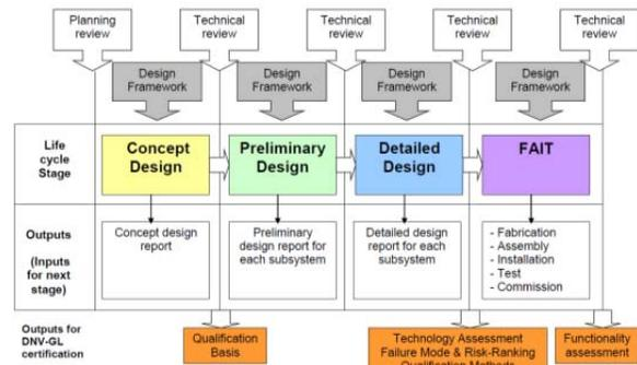
**FIGURE 3, DESIGN FRAMEWORK USED FOR THE TDU CONCEPT DEVELOPMENT.**
