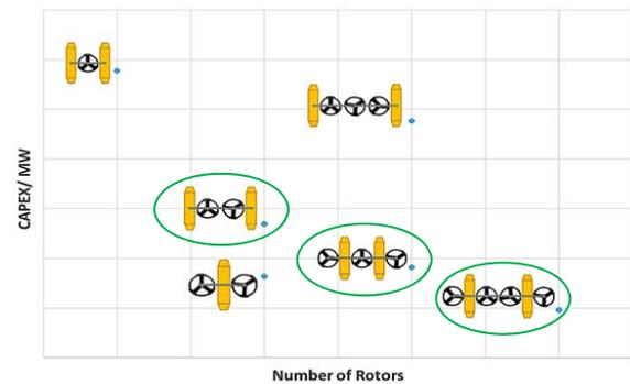
**FIGURE 4, CONCEPT EVALUATION RESULTS, SHOWING CAPEX/MW AGAINST THE NUMBER OF ROTORS FOR VARIOUS CONCEPT DESIGNS**
