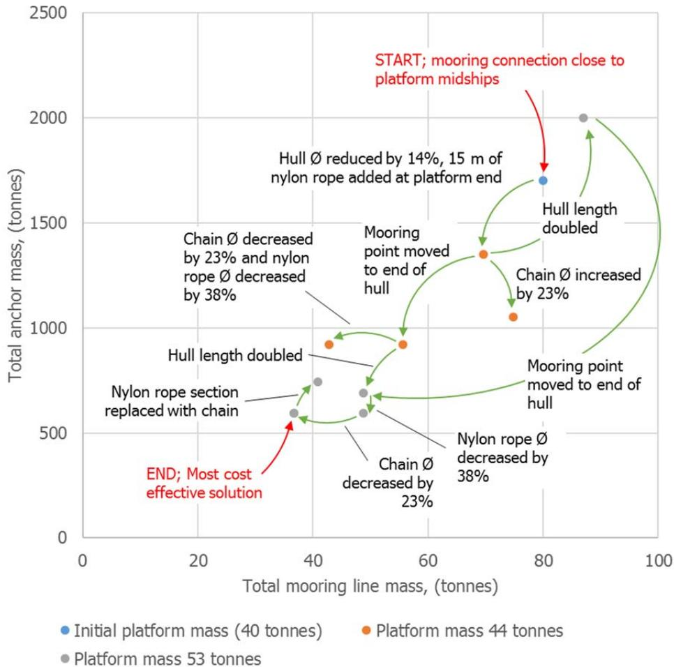
**FIGURE 6, ITERATIVE PROCESS LEADING TO PREFERRED PLATFORM AND MOORING SYSTEM DESIGN**
