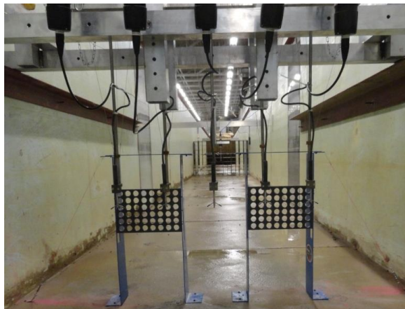
FIGURE 5. TWO POROUS PLATES INSTALLED IN THE FLUME (LOOKING UPSTREAM).
