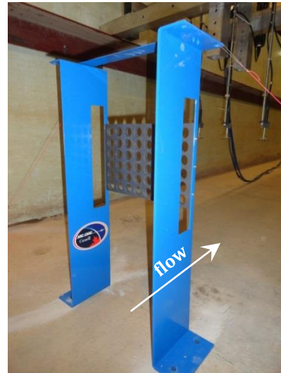
FIGURE 1. POROUS PLATE AND PLATE SUPPORT INSTALLED IN THE LWF.
