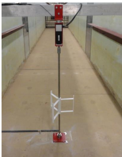
FIGURE 8. MODEL CROSS-FLOW TURBINE INSTALLED IN THE LWF (TESTS CURRENTLY ONGOING).
