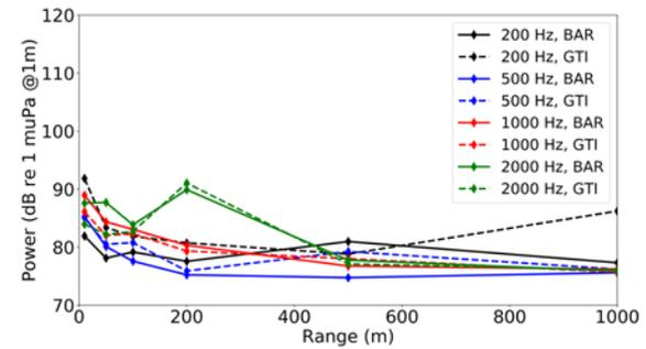
**FIGURE 3 RECEIVED SIGNAL LEVELS ON THE BAR COMPARED TO THE M20-100 VECTOR SENSOR AT VARIOUS FREQUENCIES. SIGNALS RECEIVED ON THE VECTOR SENSOR ARE COMPARABLE IN MAGNITUDE TO THOSE RECEIVED ON THE BAR, LENDING CONFIDENCE IN VSA DATA QUALITY.**
