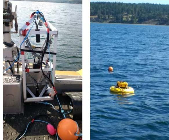
**FIGURE 1 (LEFT) VSA FRAME WITH SENSORS. GRAY FAIRING WAS USED TO MITIGATE ACOUSTIC STRUM. (RIGHT) SURFACE BUOY WITH PELICAN® CASE (HOUSING THE DATA LOGGER, VSA AMPLIFIER BOARDS, AND BATTERY PACK) STRAPPED ON.**
