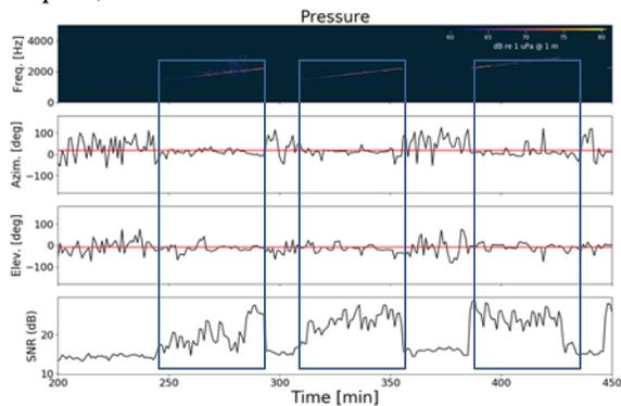
**FIGURE 5 SPECTROGRAM OF RECEIVED PRESSURE LEVELS ON THE M20-100 (UPPER PANEL), AZIMUTH ANGLE (MIDDLE PANEL) AND ELEVATION ANGLE (BOTTOM PANEL). RED LINES INDICATE TRUE AZIMUTH AND ELEVATION ANGLES. BLUE BOX SHOWS WINDOWS OF ACTIVE TRANSMISSION.**
