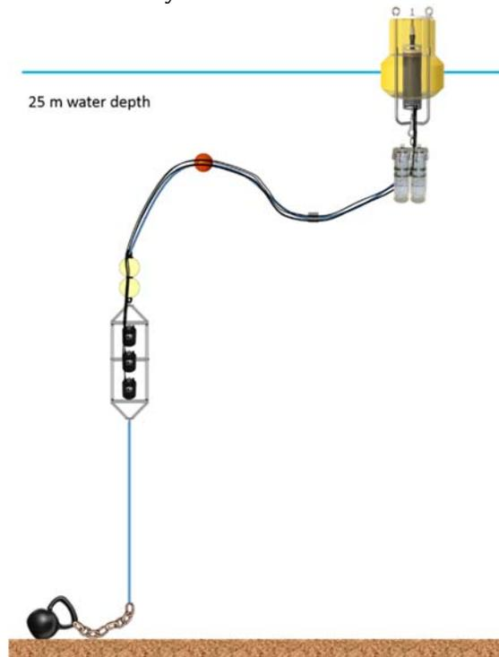
**FIGURE 2 VSA MOORING SCHEME WITH ALUMINUM ARRAY FRAME ENCLLOSING THREE VECTOR SENSORS AND THE BAR (NOT ILLUSTRATED). AN OFF-THE-SHELF DATA LOGGER AND EXTERNAL BATTERY PACK WAS MOUNTED TO THE SURFACE BUOY.**
