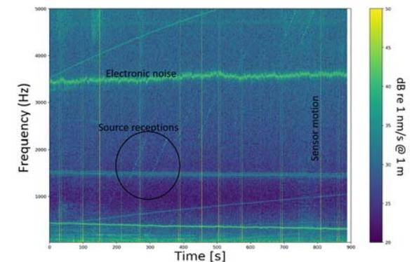
**FIGURE 4 PARTICLE VELOCITY IN THE Z-DIRECTION, MEASURED BY THE M20-100. THE LOW-FREQUENCY PULSED SINUSOIDS BETWEEN 100 HZ AND 5 KHZ AS TRANSMITTED BY THE CONTROLLED LOW-FREQUENCY SOURCE ARE VISIBLE. ALSO SEEN ARE BROADBAND STRIATIONS (VERTICAL LINES), INDICATIVE OF ARRAY MOTION AND ARTIFACTS FROM DATA LOGGER SELF-NOISE (HORIZONTAL STRIATIONS).**
