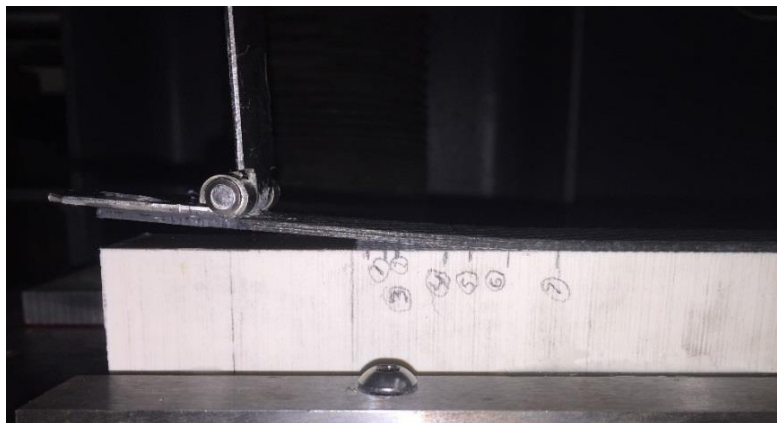
Figure 1: Single Cantilever Beam Test
