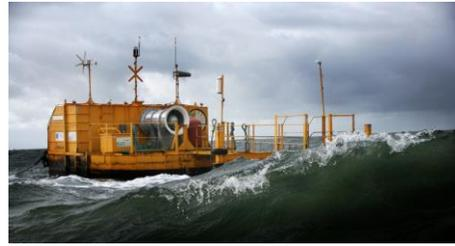
FIGURE 3. OE BUOY DEPLOYED AT ¼ SCALE GALWAY BAY TEST SITE. (TRL 5-6)
