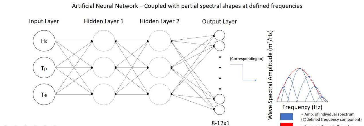
**FIGURE 1. ARTIFICIAL NEURAL NETWORK TOPOLOGY FOR PREDICTION OF SPECTRAL SHAPE FROM SUMMARY WAVE PARAMETERS**
