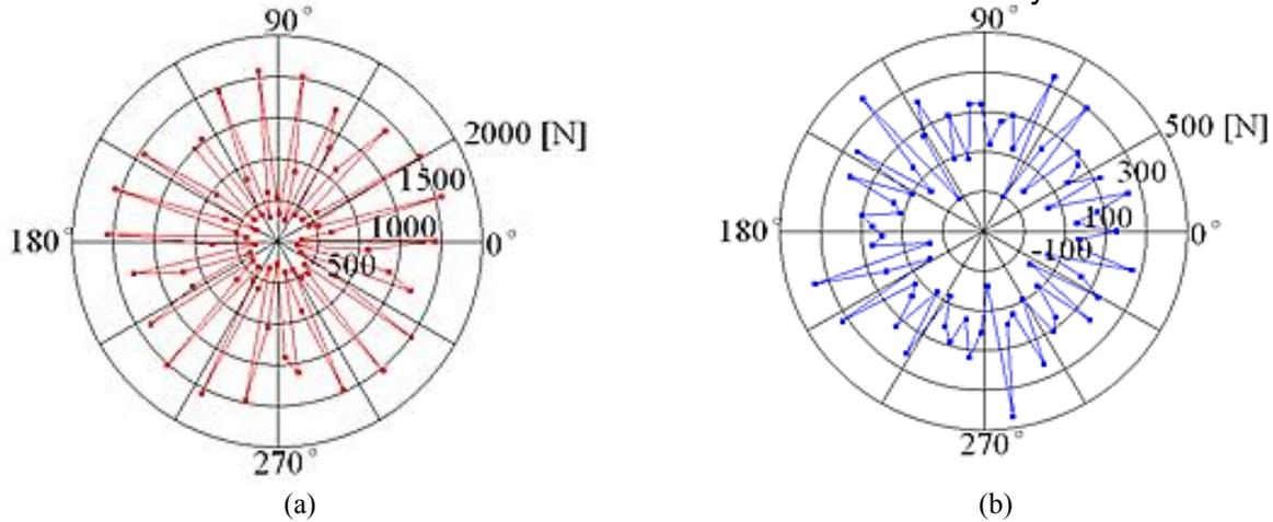
**FIGURE 2 FINITE ELEMENT ANALYSIS OF CALCULATED FORCES APPLIED TO THE RODS PASSING THROUGH CAGE ROTOR AS THE ROTOR WITH HIGHEST FORCE VALUES, (A) TANGENTIAL FORCES AND (B) RADIAL FORCES.**
