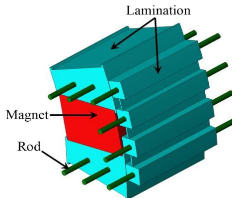
FIGURE 1. LAYOUT OF THE INNER AND CAGE ROTOR LAMINATIONS
