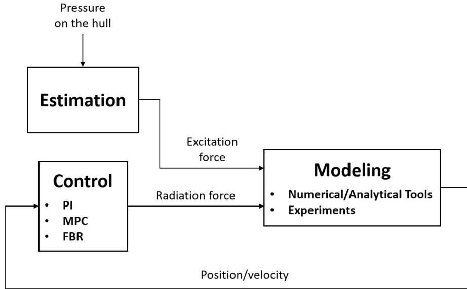
Figure 1: Block diagram showing the three main parts (modeling, estimation, control) investigated in the Advanced WEC Dynamics and Controls project of Sandia National Laboratories.
