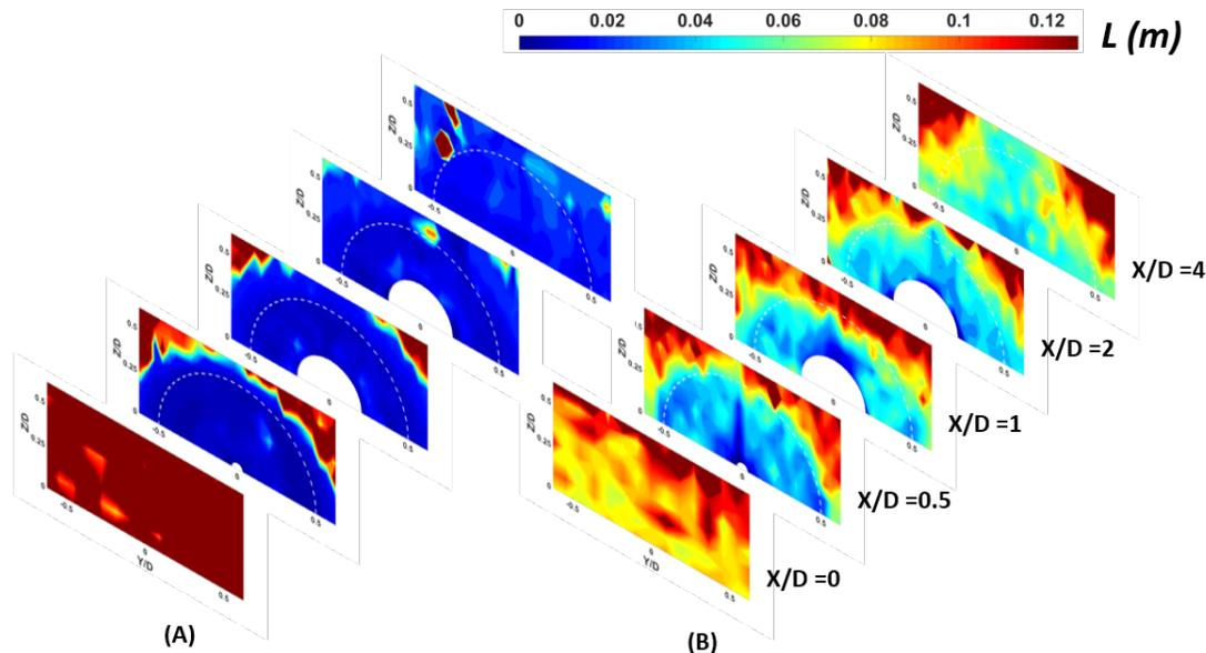
FIGURE 1. DOWNSTREAM EVOLUTION OF INTEGRAL LENGTH SCALES (A)  $Ti = 2.2\%$ , (B)  $Ti = 12.6\%$
