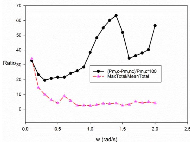
FIGURE 2. RESULTS FOR TWO WECs. The two WECs are located along the wave propagation direction, and the gap distance between them is 20 m. MaxTotal/MeanTotal is the ratio of the peak power and mean power produced by the arrays.
