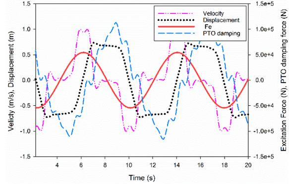
FIGURE 1. MOTIONS AND FORCES UNDER CONTROL WITH CONSTRAINTS. REGULAR WAVE WITH AMPLITUDE  $A = 0.5$  m AND FREQUENCY  $\omega = 0.8$  rad/s. CONSTRAINTS ARE  $z_{max} = 1$  m,  $v_{max} = 1$  m/s,  $K_{PTO} = 0$  N/m.
