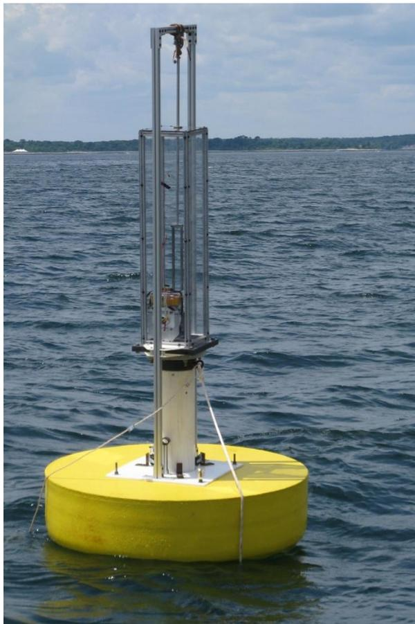
**FIGURE 3. THE UNH STUDENT WEC OFF PORTSMOUTH NH. THE PTO MOUNTED ON TOP OF THE SPAR IS PROTECTED BY A CLEAR PLASTIC HOUSING. (THE SLACK LINES LEADING OVERBOARD ARE TAG LINES USED IN THE LAUNCHING AND RECOVERY PROCESS.)**
