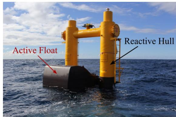
Figure 1: The Azura prototype device deployed in Hawai'i.
