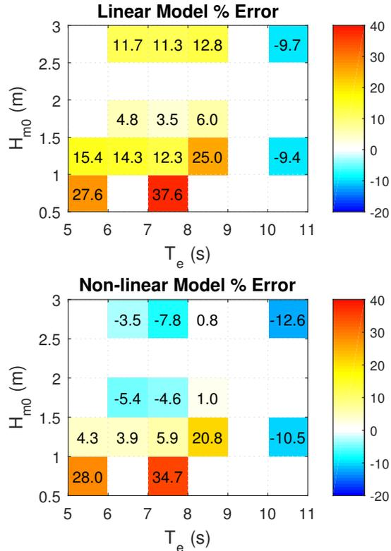
**Figure 3: Power matrix showing percent difference between WEC-Sim electrical power capture and mean experimental power capture. A positive value indicates the WEC-Sim model over-predicted power produced.**
