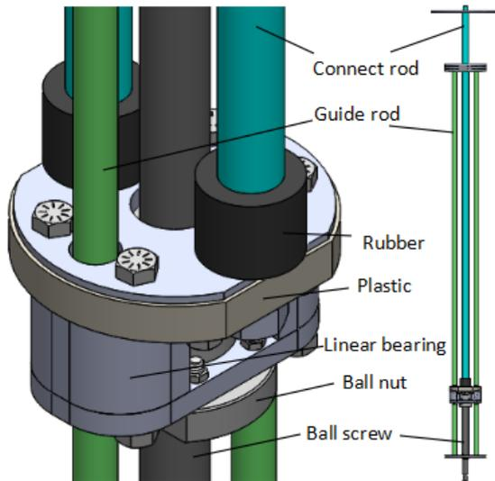
**Figure 8.** Design of nut converter
