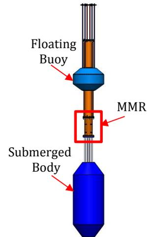
Figure 7. Overview of two-body wave energy converter with ball screw based mechanical motion rectifier.
