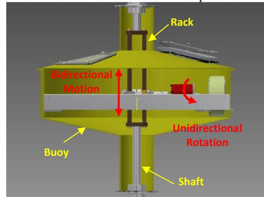
**Figure 2.** Overall design of single body wave energy converter with rack pinion based MMR.
