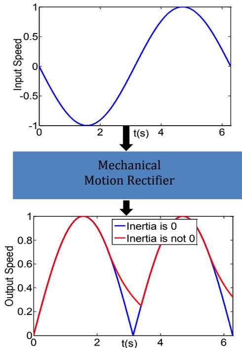
**Figure 1.** Working principle of mechanical motion rectifier. The bidirectional input motion is converted into unidirectional output rotation through two one-way bearing.
