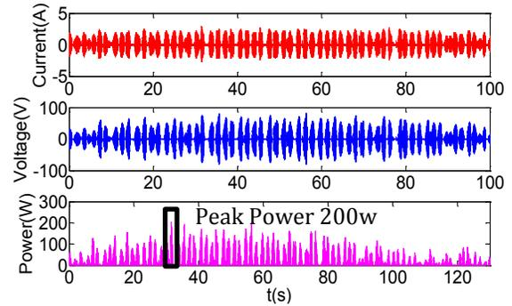
Figure 6. Ocean test of the single body wave energy converter with MMR.
