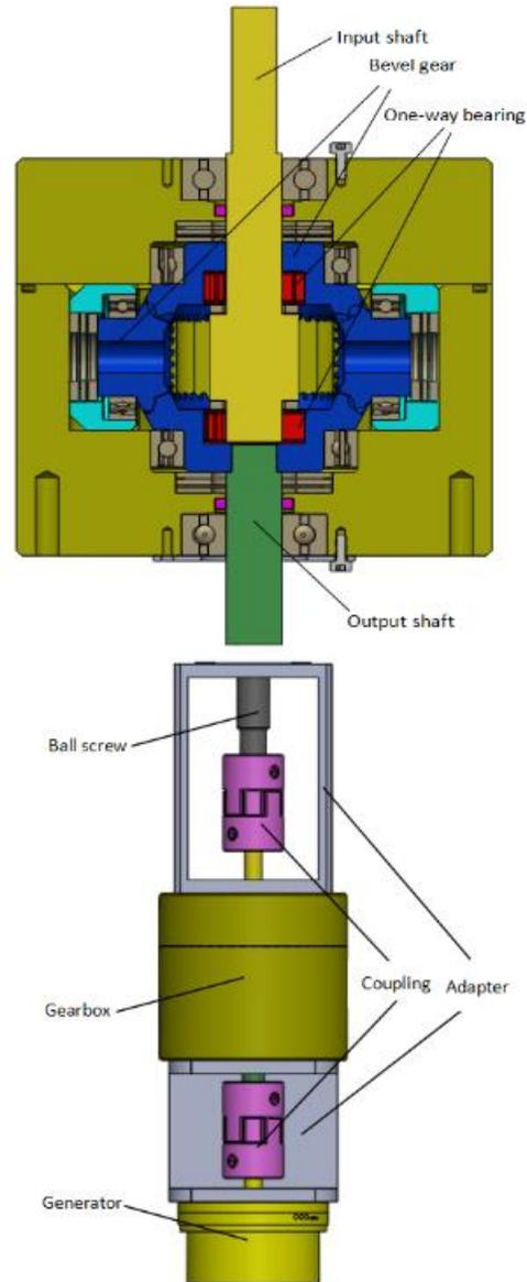
**Figure.9** Design of the gearbox
