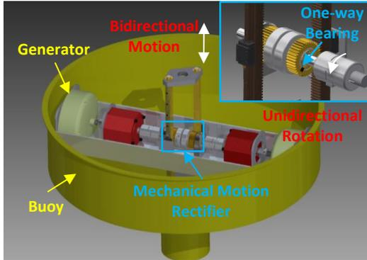
Figure 3. Detail design of single body wave energy converter with rack pinion based MMR.
