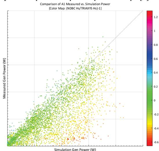
**FIGURE 2: MEASURED VS. SIMULATED GENERATOR POWER DURING THE A1 DEPLOYMENT. PERFECT MATCH WOULD FALL ON DIAGONAL LINE. COLOR SCALE INDICATES SIMILARITY OF NDBC AND TRIAXYS WAVE STATISTICS.**
