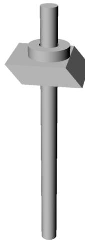
b) Symmetric Float (F1) with Spar-Plate (SP)
