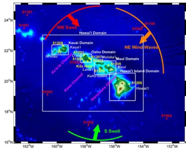
**FIGURE 2. HAWAII WAVE CLIMATE, LOCATIONS FOR OFFSHORE BUOYS (RED SQUARES) AND NEARSHORE BUOYS (YELLOW DOTS), AND MODEL COVERAGE (WHITE BOXES).**
