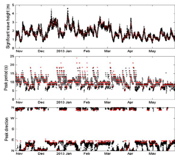
**FIGURE 3. COMPARISON OF HINDCAST AND MEASURED SIGNIFICANT WAVE HEIGHT, PEAK PERIOD, AND DIRECTION AT BUOY #51207 FROM NOV 2012 TO MAY 2013.**
