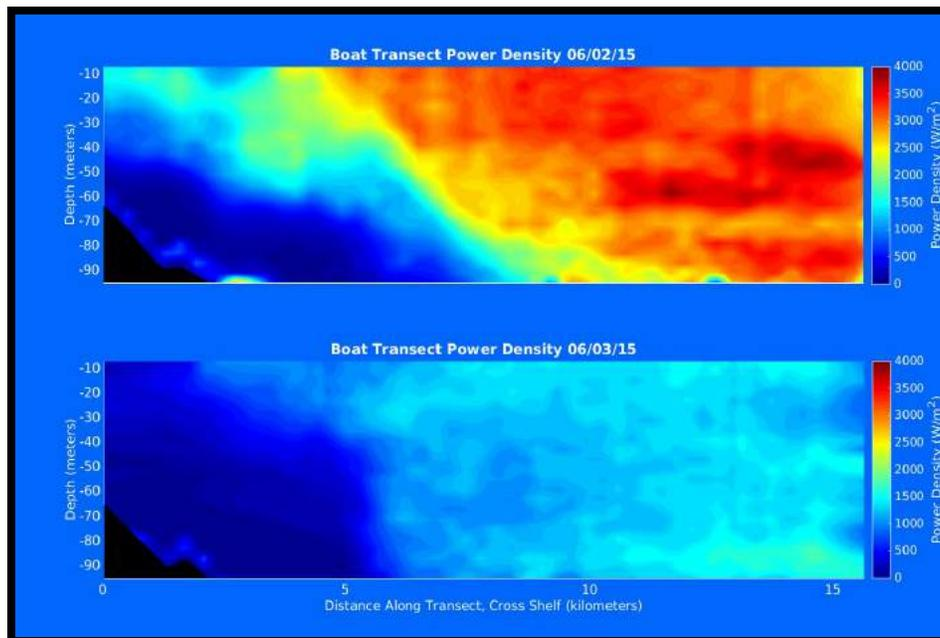
Figure 5: Power density estimates derived directly from vessel current measurements in the top 100m of the water column on two consecutive days, with distance along transect coinciding with the 100m isobath at 0 km, and proceeding offshore to the 1000m isobath at 15 km.
