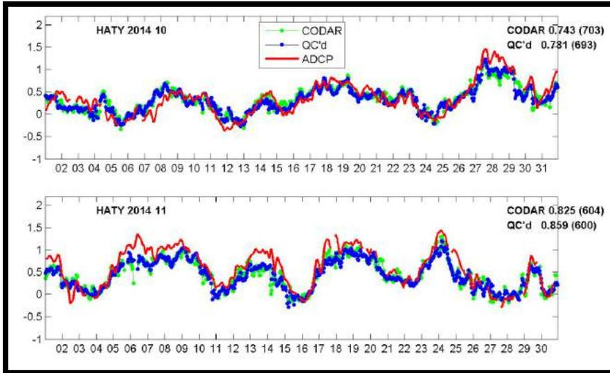
Figure 6: Comparison of the current magnitudes for the top measurement bin of the moored ADCP and the HF radar measurements for October and November of 2014. Radar vendor software produced currents are green, our QC software currents are blue, and ADCP currents 40m below the surface are in red.
