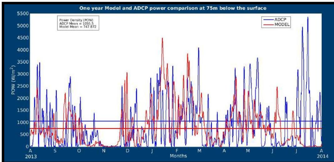
Figure 3: The model power density (red) and mooring observed power density (blue) at an assumed hub depth of 75m over a period of one year, with corresponding averages for each over the time period
