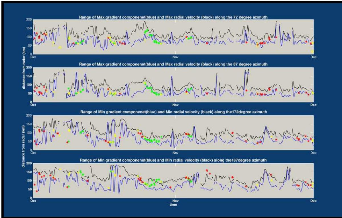
**Figure 8: Method to determine the Gulf Stream distance from the Buxton radar installation along four bearings with consistent GS coverage: distances from the radar to the maximum shear in the measured surface currents (blue) and maximum surface currents (black) provides a consistent hourly estimate of Gulf Stream location variability that is compared to available SST estimates of GS edge. SST images are ranked from 'green' for good, to 'red' for poor images.**
