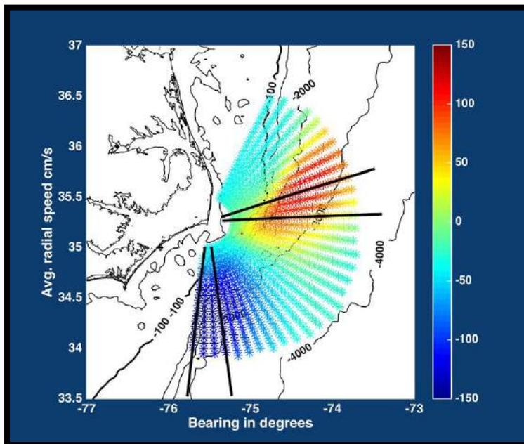
Figure 7: Hatteras HF radar map showing averaged radial current velocity magnitudes for October and November of 2014. Black lines indicate chosen bearings for Gulf Stream location analysis.
