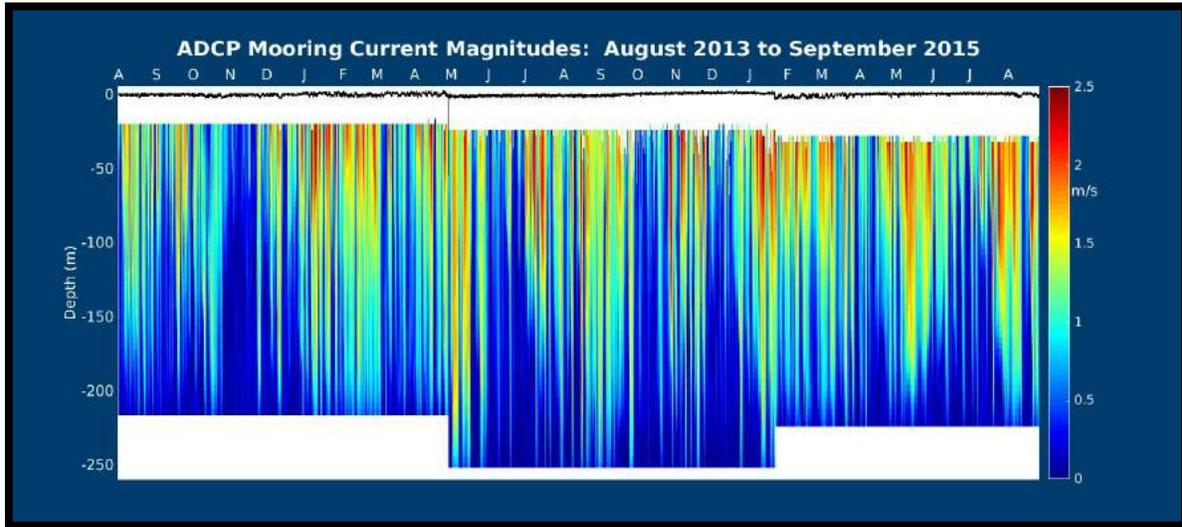
Figure 2: Current magnitudes above the moored ADCP location from August 2013 to September 2015.
