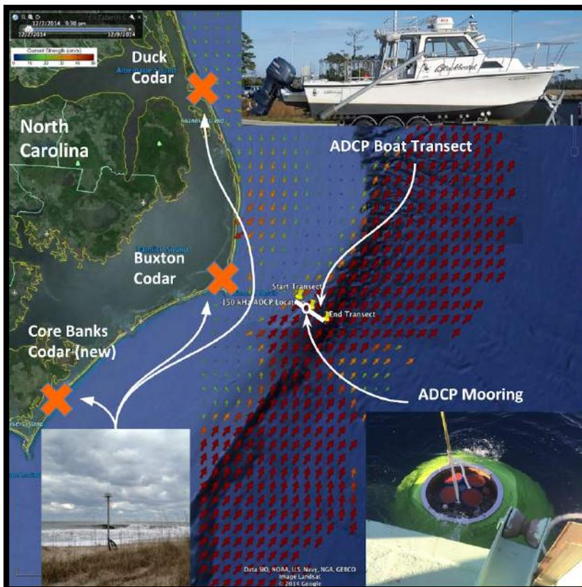
**Figure 1:** The map indicates the location of the three types of observing systems used to make current measurements. Orange 'X' marks are the locations of the 3 land-based HF radars used to measure surface currents shown in the background vector field. The yellow push pins denote the beginning of the boat transect, moored ADCP location, and end of the boat transect respectively.
