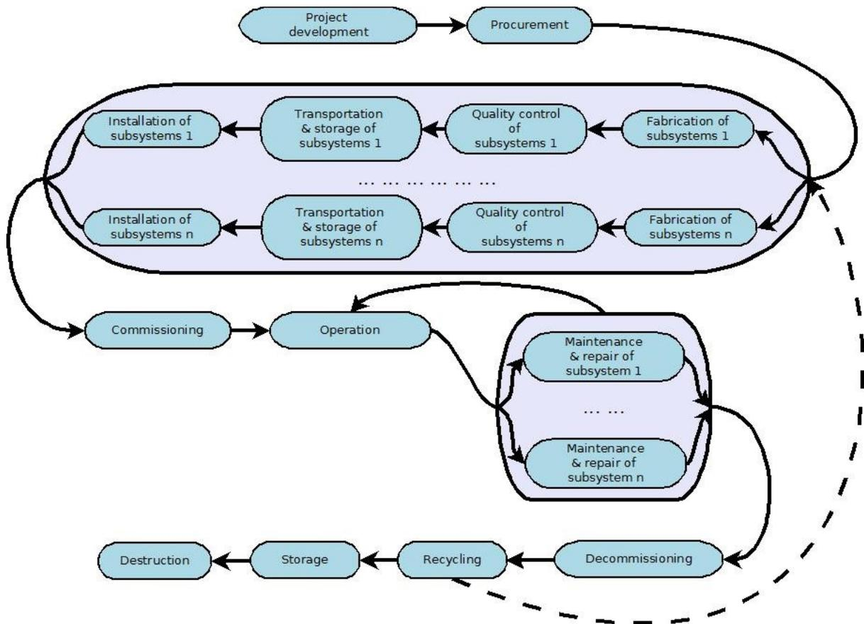
**FIGURE 4. LIFECYCLE OF A WAVE ENERGY PLANT**
