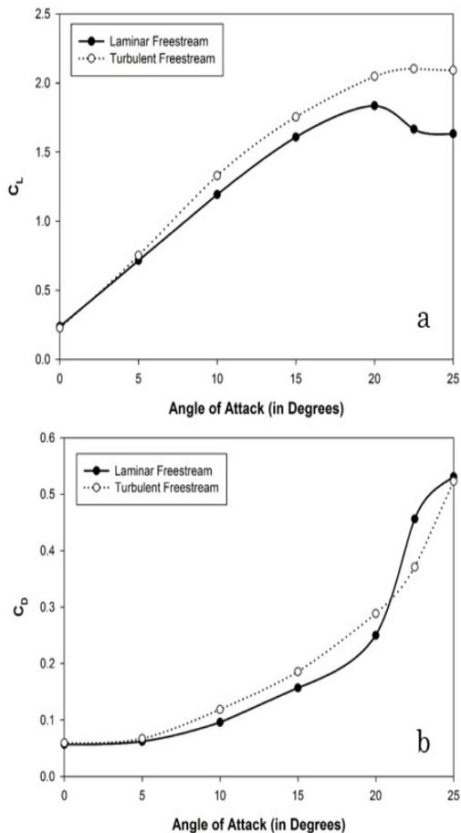
FIGURE 4. VARIATION OF (a)  $C_L$  (b)  $C_D$  WITH ANGLE OF ATTACK
