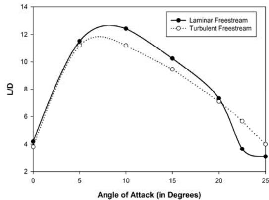
FIGURE 5. VARIATION OF L/D WITH ANGLE OF ATTACK
