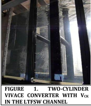
FIGURE 1. TWO-CYLINDER VIVACE CONVERTER WITH  $V_{ck}$  IN THE LTFSW CHANNEL
