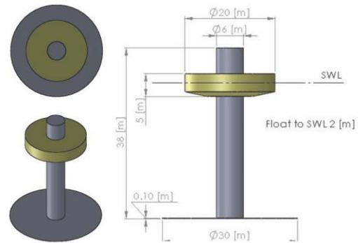
FIGURE 1. Schematic representation of the RM3 two-body point absorber [1].
