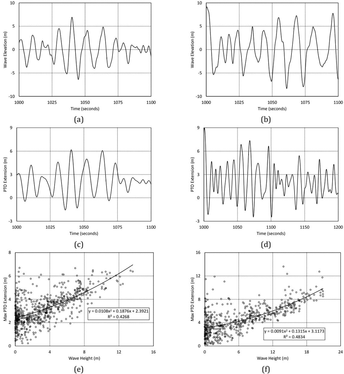
**FIGURE 2. Representative 100-sec segments from 1-hr simulations of the wave elevation process and the RM3 PTO extension for two sea states and established statistical relationship between maximum PTO extension and wave height. Plots (a), (c), and (e) are for the sea state with  $H_s = 8.2$  m,  $T_p = 11.0$  s; plots (b), (d), and (f) are for  $H_s = 16.0$  m,  $T_p = 13.3$  s.**
