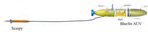
Fig. 1: Schematics of towing the SeaSPY magnetometer using an AUV
