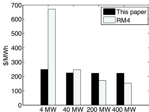
**FIGURE 4. LCOE COMPARISON WITH SANDIA RM4.**
