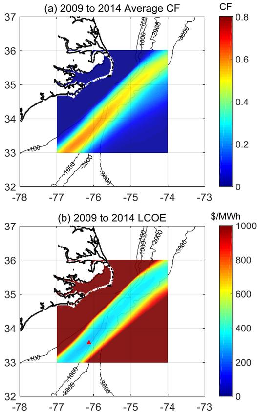
**FIGURE 2. (A) SIX YEAR AVERAGE CAPACITY FACTOR FROM 2009 TO 2014. (B) SIX YEAR LEVELIZED COST FROM 2009 TO 2014, RED TRIANGLE INDICATES LOCATION WITH MINIMUM LCOE.**
