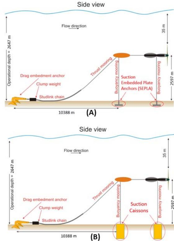
**FIGURE 7.** SIDE VIEW OF (A) FIXED AND (B) MOVABLE FOUNDATION SYSTEMS-AFTER [13].
