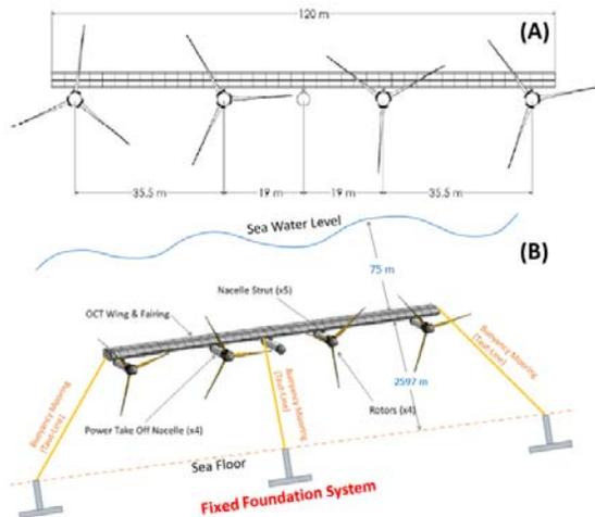
**FIGURE 6.** (A) DETAILS OF RM4 DEVICE; (B) FRONT OF MODIFIED RM4 MODEL [13].
