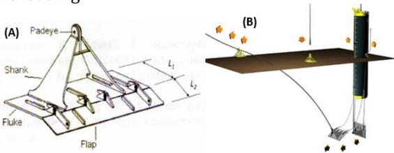
**FIGURE 3.** (A) SEPLA CONFIGURATION [10]; (B) SEPLA CONCEPT - SUCTION INSTALLATIONS, CAISSON RETRIEVAL, ANCHOR KEYING, & THE MOBILIZED ANCHOR [11].
