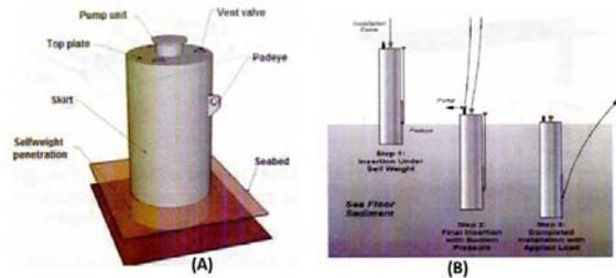
**FIGURE 2.** (A) SUCTION CAISSON CONFIGURATION ([HTTP://WWW.OFFSHOREMOORINGS.ORG](http://www.offshoremoorings.org)); (B) INSTALLATION PROCEDURE OF SUCTION CAISSON [8]
