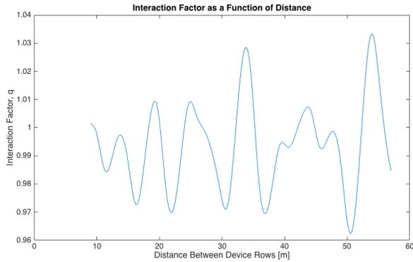
**FIGURE 3: INTERACTION FACTOR AS A FUNCTION OF DISTANCE BETWEEN ROWS FOR A 60 X 60 METER SPACE**
