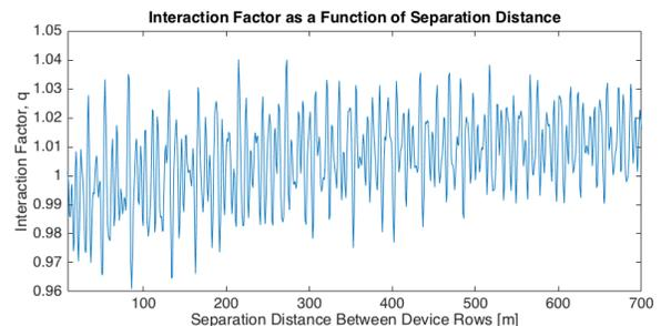
**FIGURE 7: INTERACTION FACTOR AS A FUNCTION OF DISTANCE BETWEEN OFFSET ROWS FOR A 60 X 700 METER SPACE**
