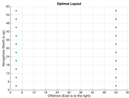
**FIGURE 4: OPTIMAL SEPARATION SPACING IN A 60 X 60 METER SPACE**
