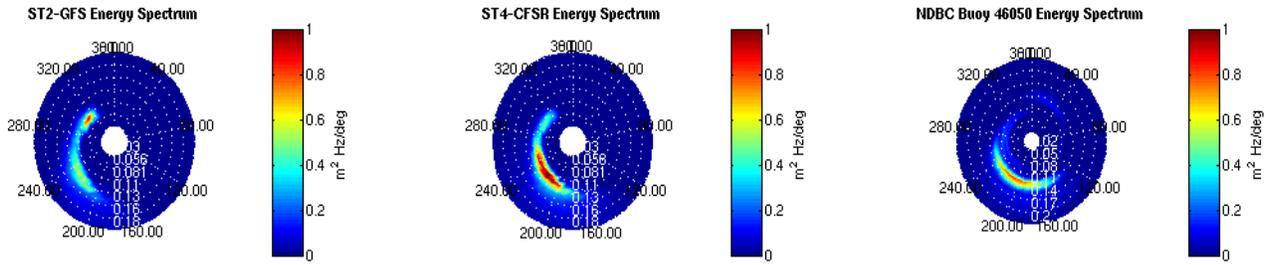
**FIGURE 4 SPECTRAL OUTPUT FOR ST2-GFS, ST4-CFSR AND NDBC BUOY 46050 NOV. 17 1700**
